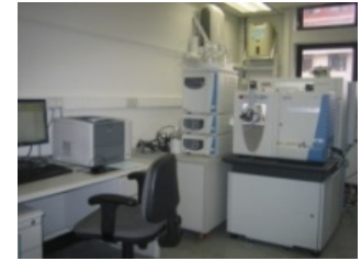
LTQ Orbitrap Velos LC/MS/MS system
