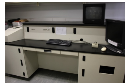
Voyager-DE STR MALDI Time-of-Flight Mass Spectrometer
