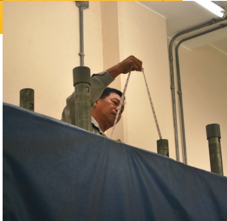
Participants conducting sonic logging test
