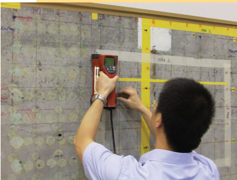
Participant conducting covermeter survey by electromagnetic covermeter
