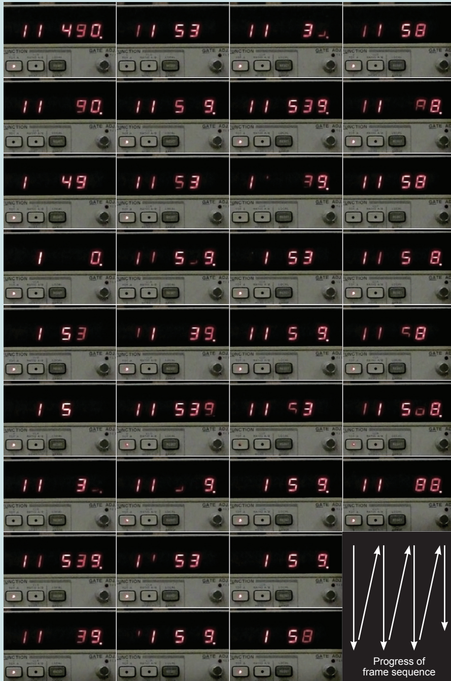
Figure 4. Display of a universal counter captured by a high speed digital camera at 420 fps or every 2.38 ms.
