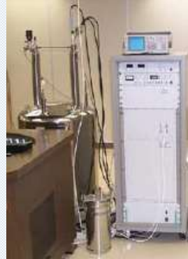
Quantum Hall Resistance Standard 量子化霍爾電阻標準
