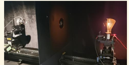
Setup for luminous intensity measurement of a light source by a reference photometer.
